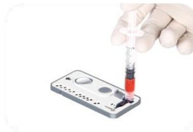
Step2: Fill the inlet with sample and slide the cap to seal the sample inlet.
